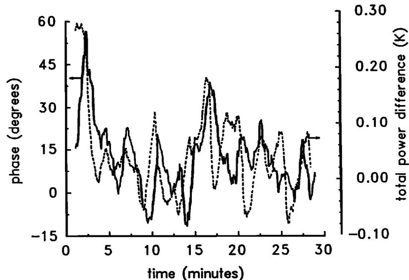
**Figure 4.** Observation 3: comparison of phase fluctuations with total power fluctuations for an observation of Jupiter on April 6, 1992. Observation was started at 2345 LT; temperature was 315 K.
