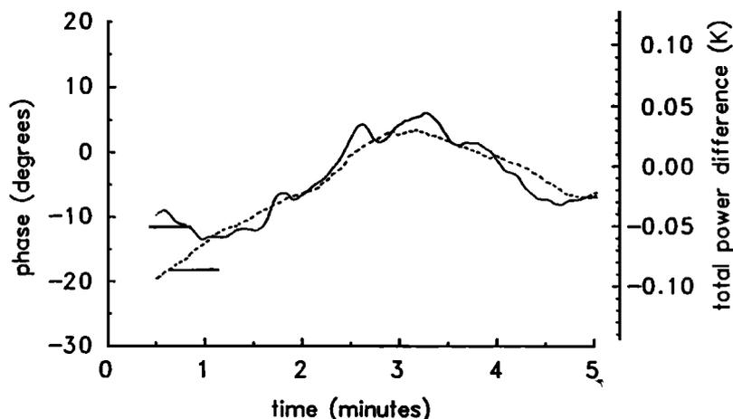
**Figure 2.** Observation 1: comparison of phase fluctuations with total power fluctuations for an observation of Jupiter on March 18, 1992. Observation was started at 2345 LT; temperature was 320 K.
