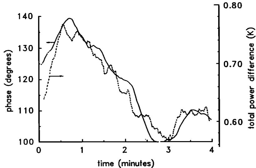
**Figure 3.** Observation 2: comparison of phase fluctuations with total power fluctuations for an observation of Mars on May 22, 1992. Observation was started at 1700 LT; temperature was 324 K.
