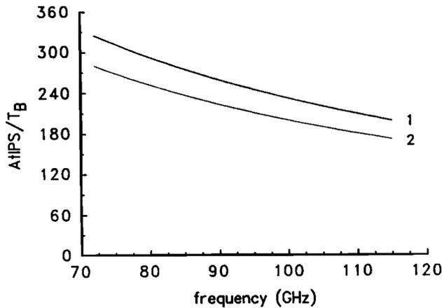
**Figure 1.** Comparison of  $\phi/T_w$  calculated with and without the assumption that the atmospheric temperature is constant in regions where the water vapor density has significant values. The temperature on the ground is 287 K and the water vapor density on the ground is  $5 \times 10^{-3} \text{ kg/m}^3$ . Curve 1, calculation with approximation; and curve 2, calculation without approximation.
